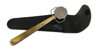
The **ASME MAGNETIC FIELD INDICATOR** is used as a convenient rough check of the adequacy and direction of part magnetization. It is not used as quantitative of fields strength or distribution and reflects only field strength and direction at the surface and in the area of the part under test.
